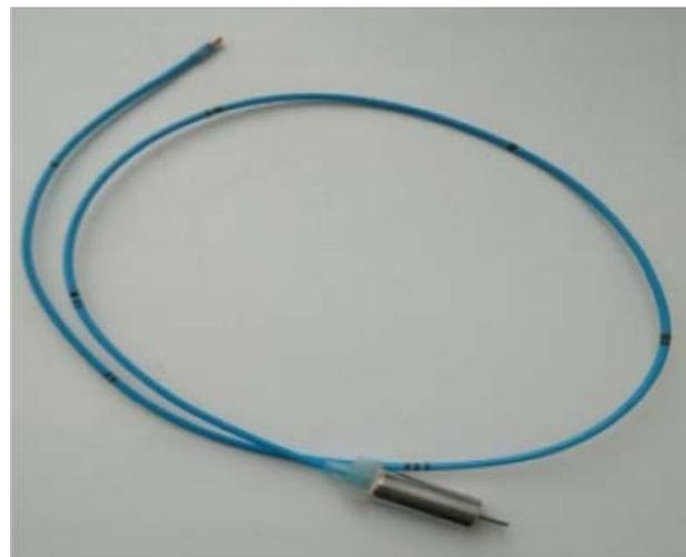
Figure 1. **Bipolar single-shaft electrode**
